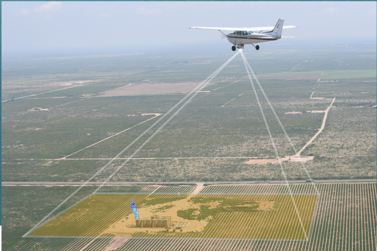
American Patrols (AP) conducting a Bridger Photonics field survey. Supplemental graphics depict the survey scan area (orange) and identified methane emissions (blue). Graphic depiction to demonstrate the technology and does not represent results from a facility survey. Photo credit: AP
